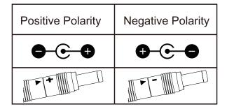
Depending on the device, the orientation of the positive and negative poles in the depiction may be reversed but, if the device requires positive polarity, the symbol will be on the side with the C shaped arc. If negative polarity is required, the + symbol will be on the side with the C shaped arc.
